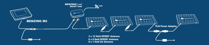
The system can be extended to a maximum of 8 PLB Speed<sup>2</sup> or G2 Antennas at any time using the **PLB Power Adapter.**
